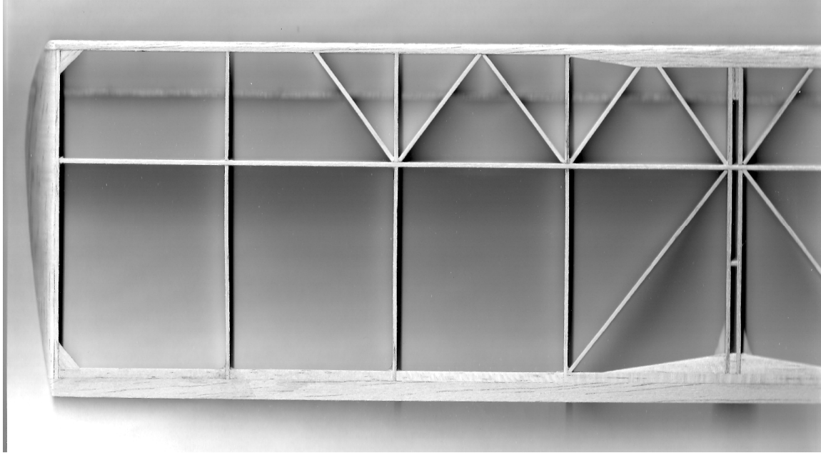
Top Banana 200 stab bottom, note 2-piece TE and limit of diagonal ribs
