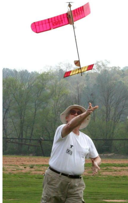
Dohrman testing wing spars on his new E-36--note stab position
