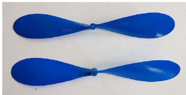
And here's one I prepared earlier! This is a standard 150mm Union prop which started at 3.2g and finished at 1.6g. You can go a lot lighter for indoor.
